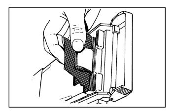
Close the camera back and rotate its latching cover, making sure the black paper tab is outside the camera back.
